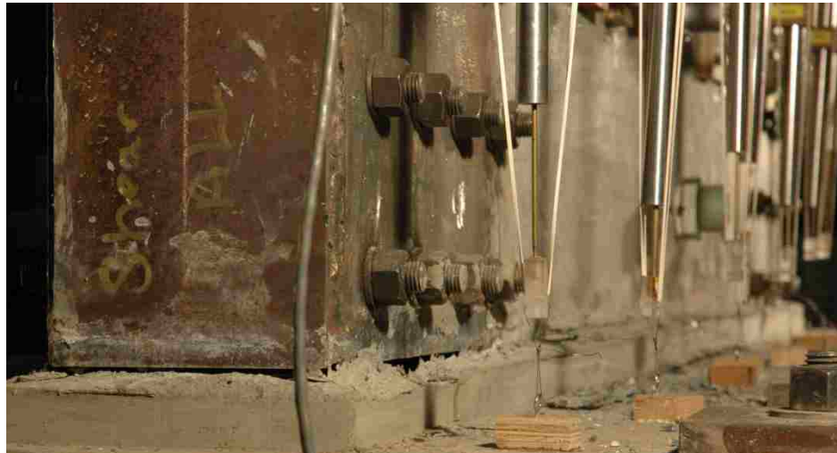
Figure 6-4 - Plate-confined Wall at 1% Roof Drift
