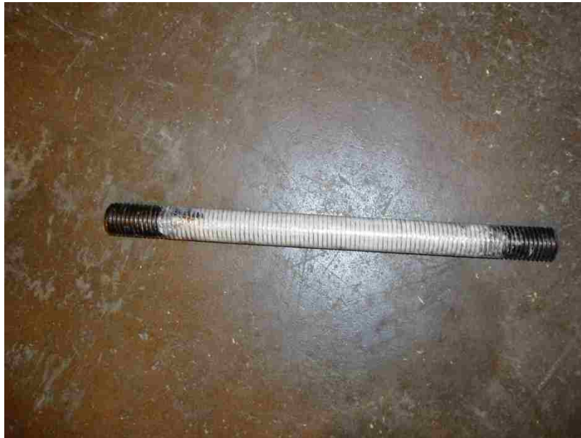
Figure 4-5 – Confinement Bolt Debonded with Grease and Plastic Wrap
